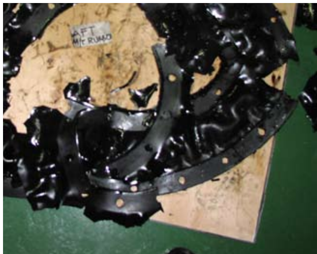
Defective rubber membranes may cause severe engine damage.
