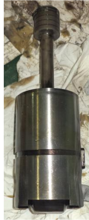
EXHAUST ROLLER AT DISMANTLED CONDITION(FOR REFERENCE ONLY) MEASUREMENT CAN BE TAKEN ON THE TOP OF THE PISTON WITHOUT REMOVING OIL CYLINDER AND ROLLER
