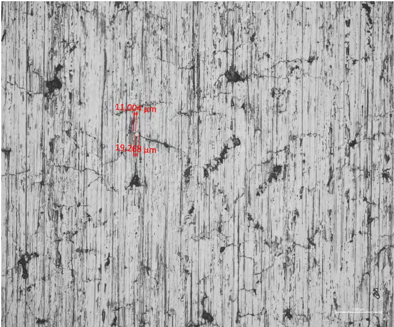
Observations: Cylinder scuffing with partially developed network of micro-cracks. A few visible cat fines.
